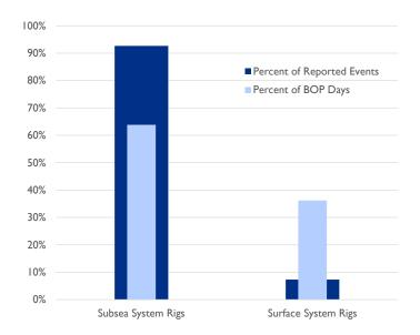
**NOTE**: Subsea system rigs represented include drillships, semisubmersibles, and dynamically positioned (DP) semisubmersibles. Surface system rigs represented primarily include platform rigs and jackups. **SOURCE**: U.S. DOT, BTS, SafeOCS Program.
