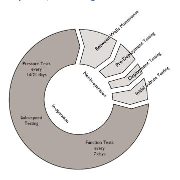
**KEY:** In-operation Not-in-operation **NOTE:** The figure illustrates the cyclical MIT regime practiced on subsea WCE systems, scaled to show the approximate time split for an average new well.
